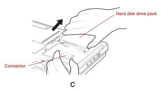
Figure 3-20 Removing the hard disk drive pack
